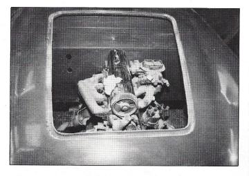
Austin Healey 100/4. The chassis for the car is a fairly rudimentary twin rail ladder item with cross bracing. It takes Ford engines and gearboxes, and by the look of the engine bay, there seems to be enough room to put in the 3 litre V6 or maybe the Rover V8. The
