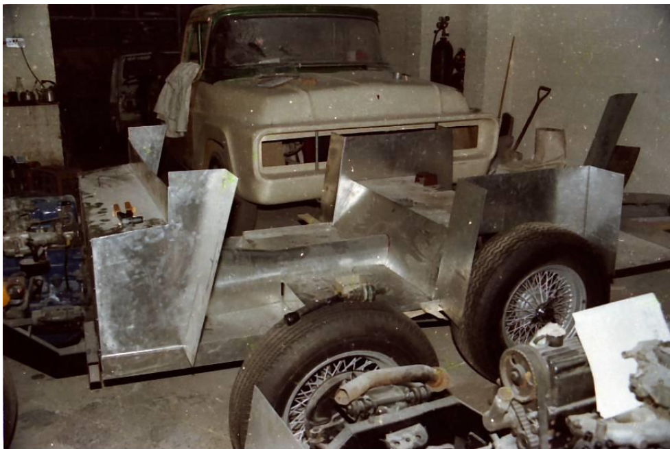
Clearly visible the chassis design and the panelling of floor and scuttle area. In the foreground the chassis with Vauxhall Chevette front axle and Ford Pinto engine. Chassis designed by PCF Motors.
