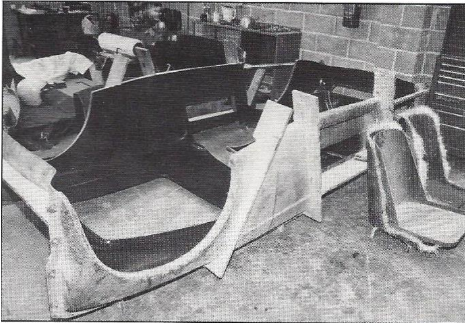
The production moulds for an Austin-Healey 100/4 replica by Pete Farries.
